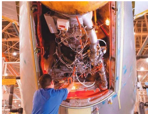
APU Insulation System Installed
